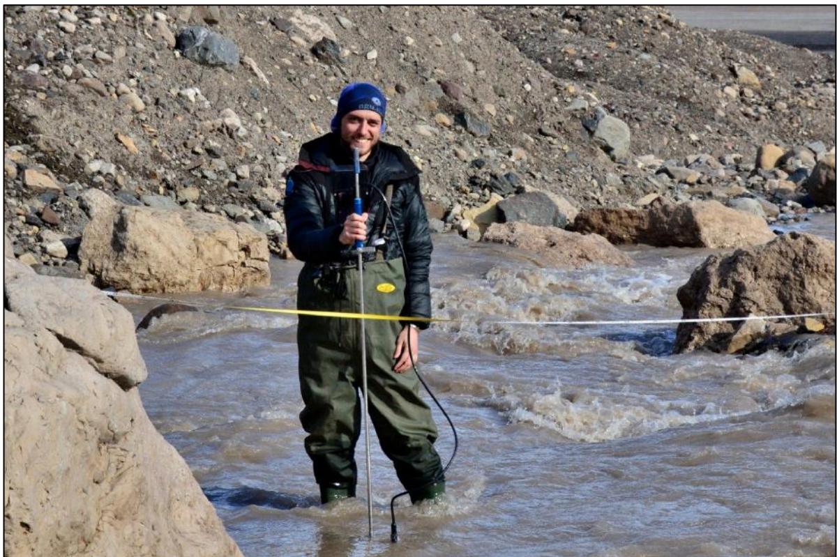
Fig. 3.3.1. Jakub Malecki measuring discharge on Sven river (July 20 th 2012).
