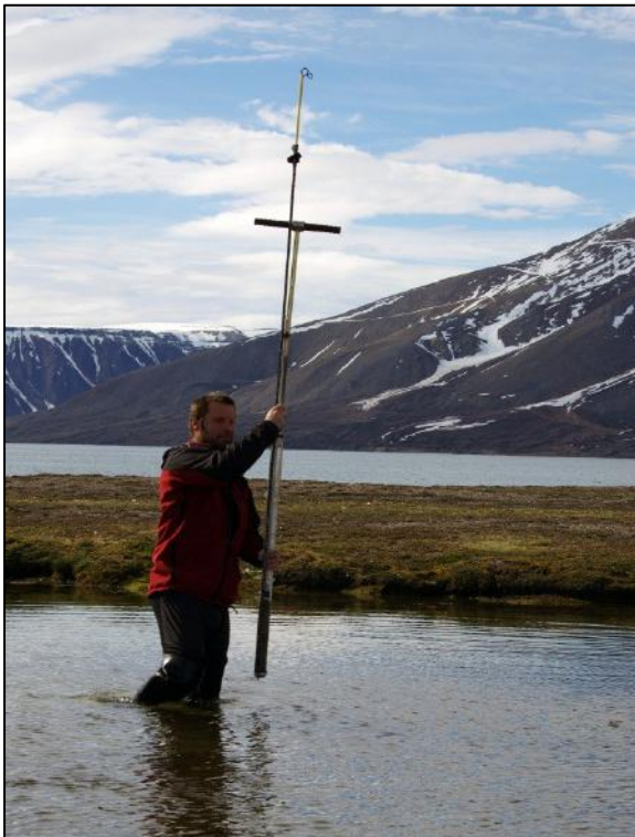
Fig. 3.4.3. Sampling the lake sediments for the study of ancient cyanobacteria.
