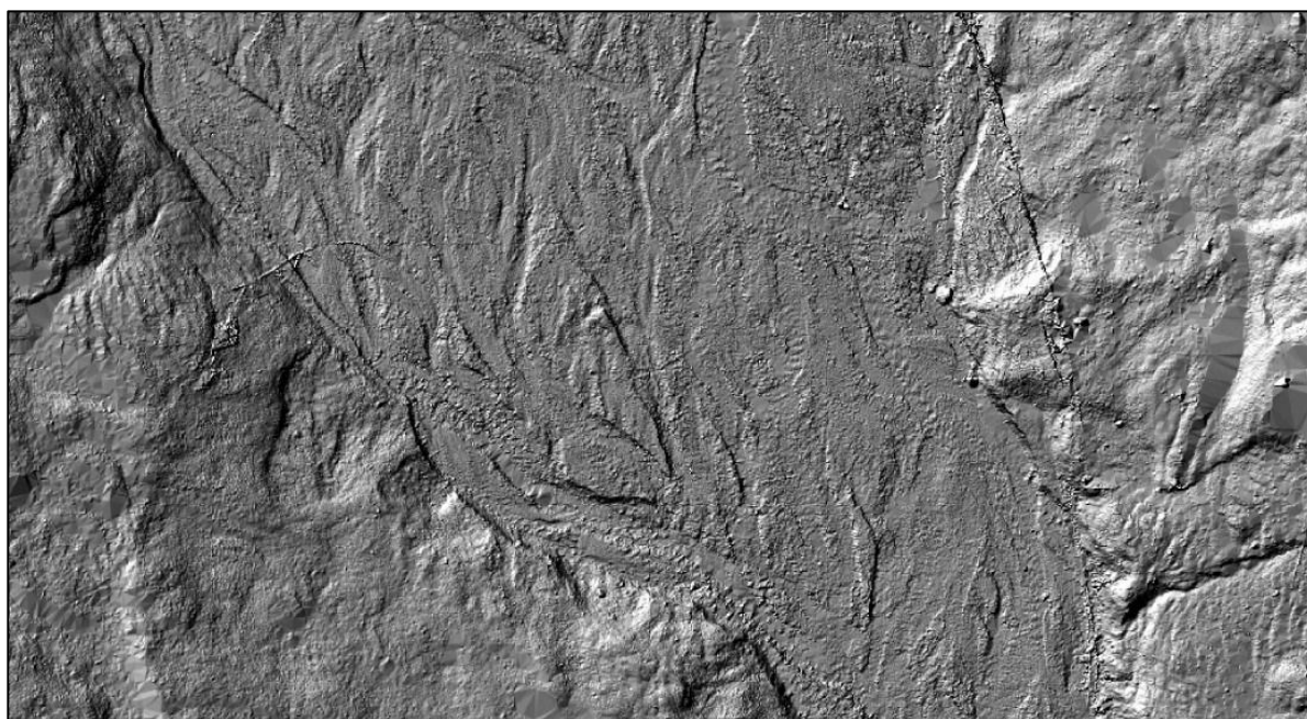
Fig. 3.1.1. DEM of Bertilbreen outwash plain produced by laser scanning.
