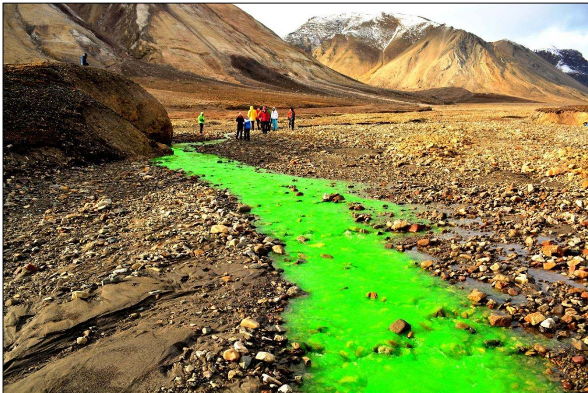
Fig. 3.3.1. Discharge monitoring on Ferdinand using uranine dye tracer method.
