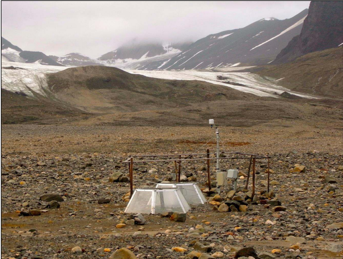
Fig. 3.3.3. Automatic weather station (AWS3) complemented with the Open Top Chamber system providing both local climate and microclimate data on the foreland of Hørbye Glacier.
