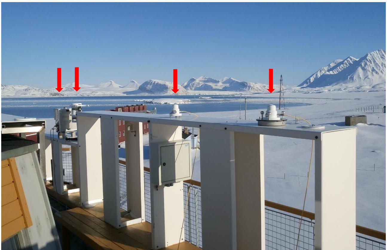
Figure 2. Mounting of instruments participating in the UV-ICARE inter-comparison campaign. Instruments marked by red arrows (from left to right): UV-RAD, GU, UVS-E-T IGF-PAS, UVS-E-T Univ. South Bohemia.
