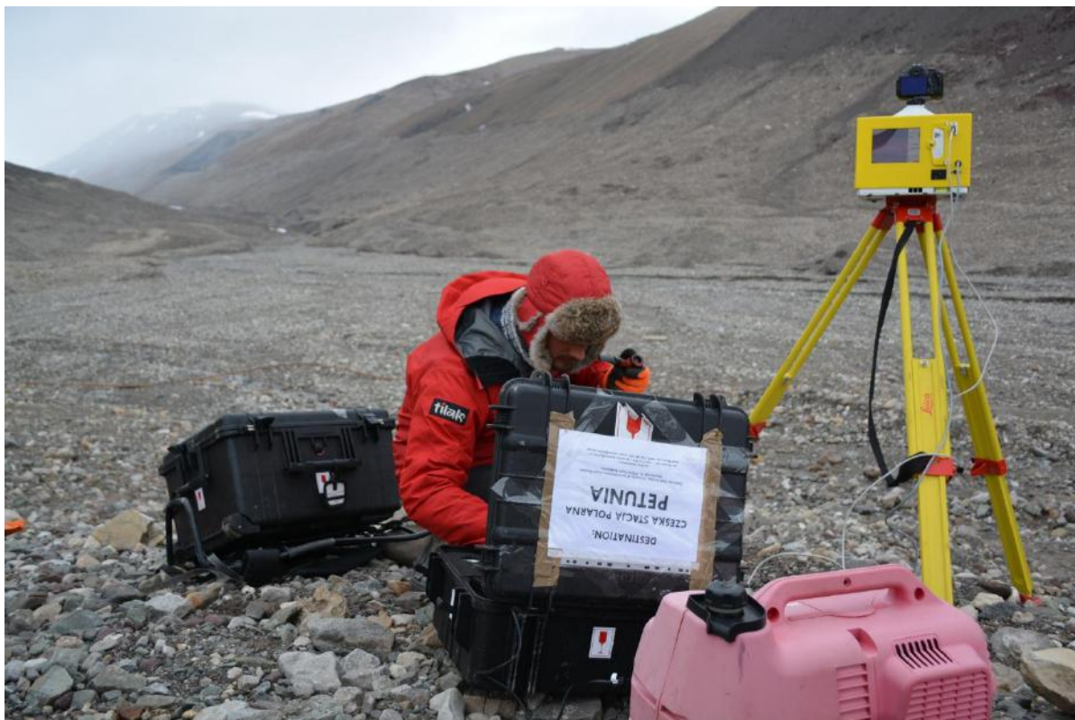
Fig. 3.1.1. Laser scanning on Bertilbreen outwash plain.
