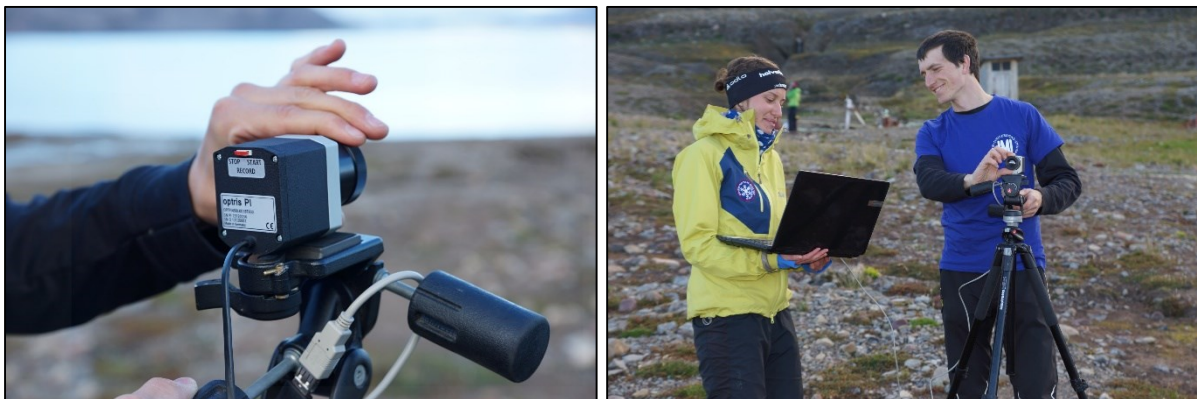
Fig. 2.2.6. Measurements of surface temperature in the coastal area of Petuniabukta by the OPTRIS infrared camera system.
