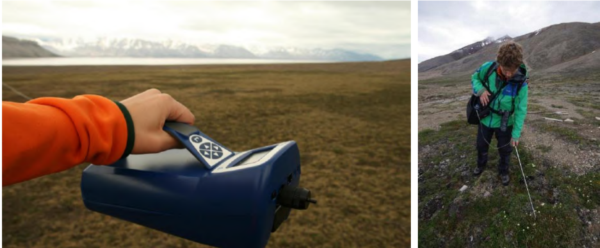
Fig. 2.2.5. Measurements of ultrafine particles by P-track instrument in the coastal area of Petuniabukta.
