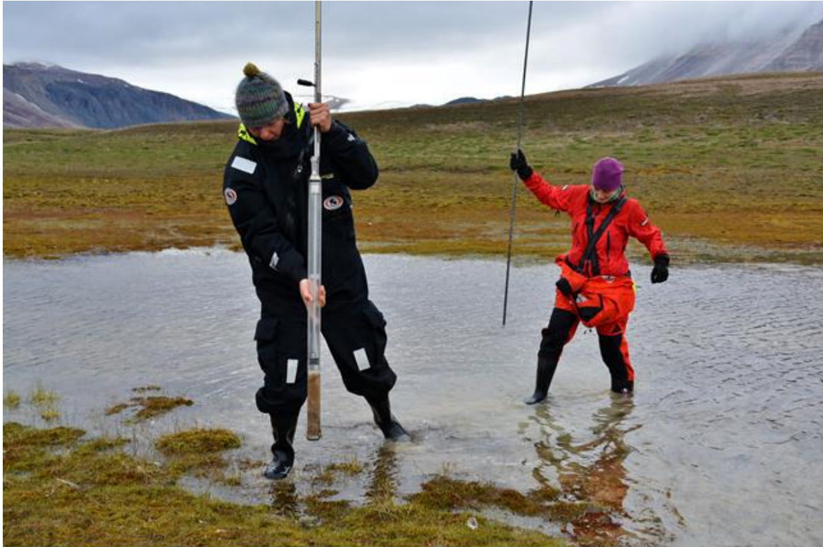
Fig. 2.3.3. Taking sediment core from the shallow marshes in Ebbadalen.
