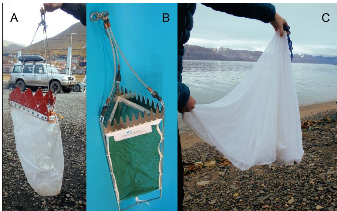
Fig. 2.3.6. Collecting tools: (A) homemade triangular dredge, (B) professional triangular dredge sold by KC Denmark A/S company, (C) homemade casting net.
